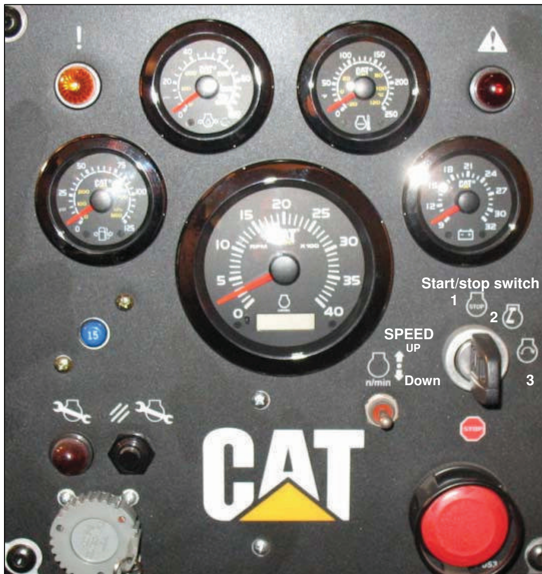
Figure 4-5: Layout diesel control panel
